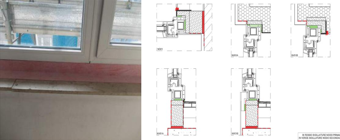
The image shows a photograph of a window frame on the left and five technical cross-section diagrams on the right. The diagrams are labeled IN01, INV01A, INV01B, INV01A, and INV01B. A legend at the bottom right indicates: IN ROSSO SIGILLATURE NODO PRIMARIO (Primary sealant node in red) and IN VERDE SIGILLATURE NODO SECONDARIO (Secondary sealant node in green).
